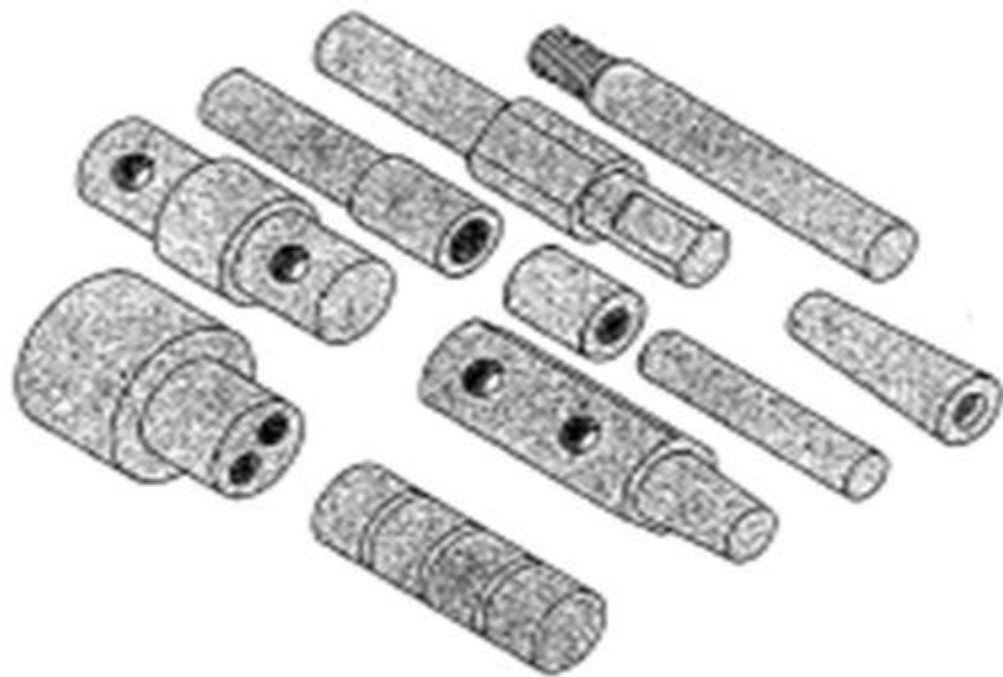
Figure 15.2 A family of parts with similar manufacturing process requirements but different design attributes. All parts are machined from cylindrical stock by turning; some parts require drilling and/or milling.
