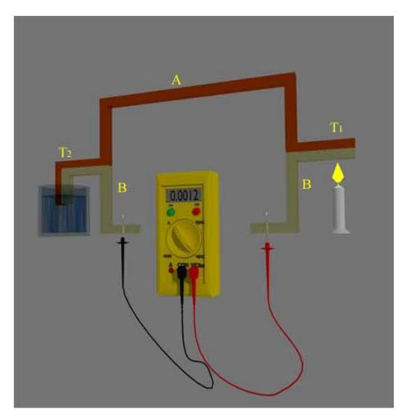
In thermocouple temperature sensor, the temperature of hot junction is measured in respect of cold junction. The thermoelectric potential is generated in thermocouple instrument is in range of  $\mu$ V. Hence, the voltmeter connected to measure the thermoelectric potential is extremely sensitive and the temperature can be read directly from this voltmeter, if it is calibrated properly in the scale of temperature.
